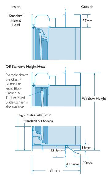
Note: High Profile Sill to be used where >300 Pa Water Ratings are required. 102mm louvres are not suitable for Easyscreen<sup>™</sup> Window Systems using the High Profile Sill as the blades controlled by the bottom handle will only open to 28°
