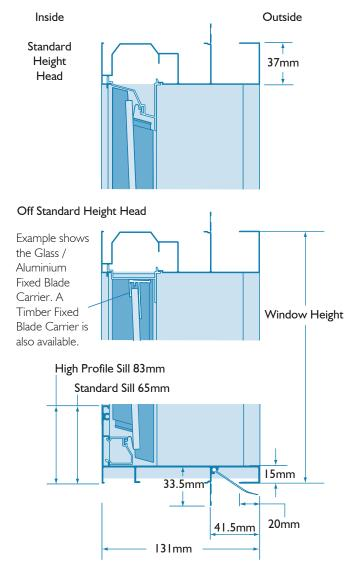
Note: High Profile Sill to be used where >300 Pa Water Ratings are required. I 02mm louvres are not suitable for Easyscreen™ Window Systems using the High Profile Sill as the blades controlled by the bottom handle will only open to 28°
